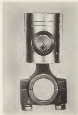
4-2. The assembled piston, piston pin, lock pin and the connecting rod. Note that two cap screws instead of two bolts are used at the crank end of the connecting rod. (General Electric Co.)
